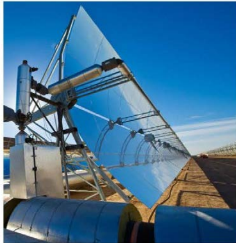
Parabolic Trough Collector
